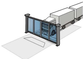
Truck arrives. An open pulse is given by the access control system. The Speedgate opens when loops, photocells and laser indicate that it is safe to do so.
