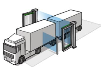
Truck passes the Speedgate. The laser supplements the photocells here, in particular ensures that the drawbar is detected at all times.
