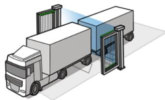
Truck passes the Speedgate. The laser supplements the photocells here, in particular ensures that the drawbar is detected at all times.
