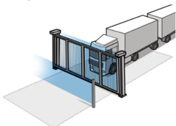
Truck arrives. An open pulse is given by means of the access control system. The Speedgate opens when photocells and laser indicate that it is safe to do so.
