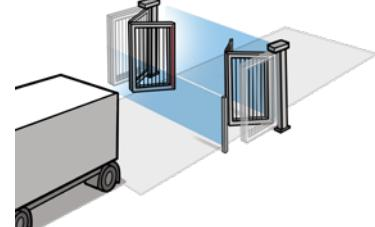
Immediately after the Truck has passed the second laser and all safeties have been released, the Speedgate closes quickly. Ready for the next cycle.
