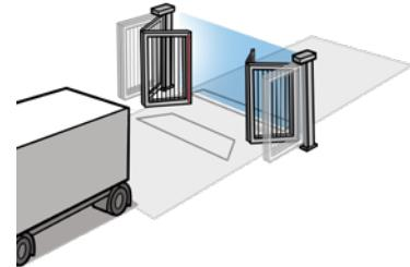
Immediately after the Truck has passed the trapezoidal loop and all safety devices have been released, the Speedgate closes quickly. Ready for the next cycle.
